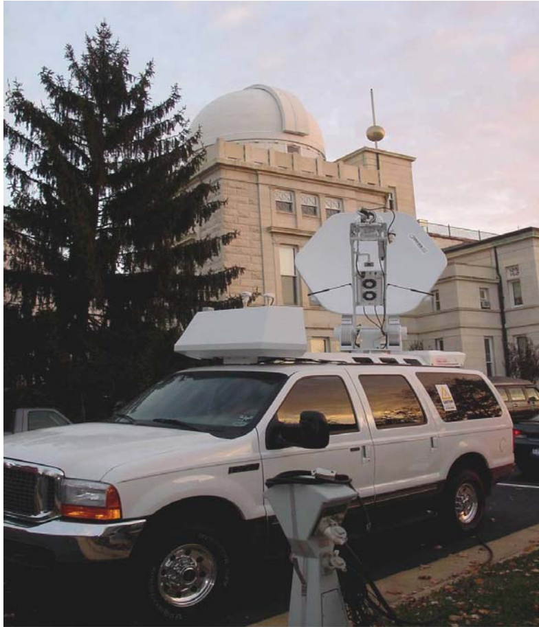
Figure 9. Mobile Earth Station for TWSTT calibration has been driven 18,000 miles this year. Small enough to be carried on a C141 military transport plane, it could be equipped to serve as a hop-link by communicating through two different satellites and/or frequencies simultaneously. Its automated pointing system makes it easy to find a satellite in the field. In the background, one can see a functional copy of the Time Ball originally built to transfer time to ships sailing up the Potomac River.
